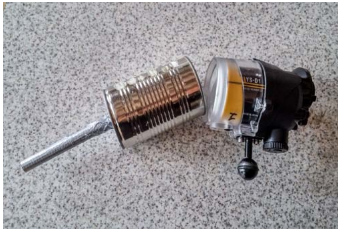
Baked bean can snoot ready to be attached to the strobe. LG G3, f2.4, 1/20, ISO 100.
