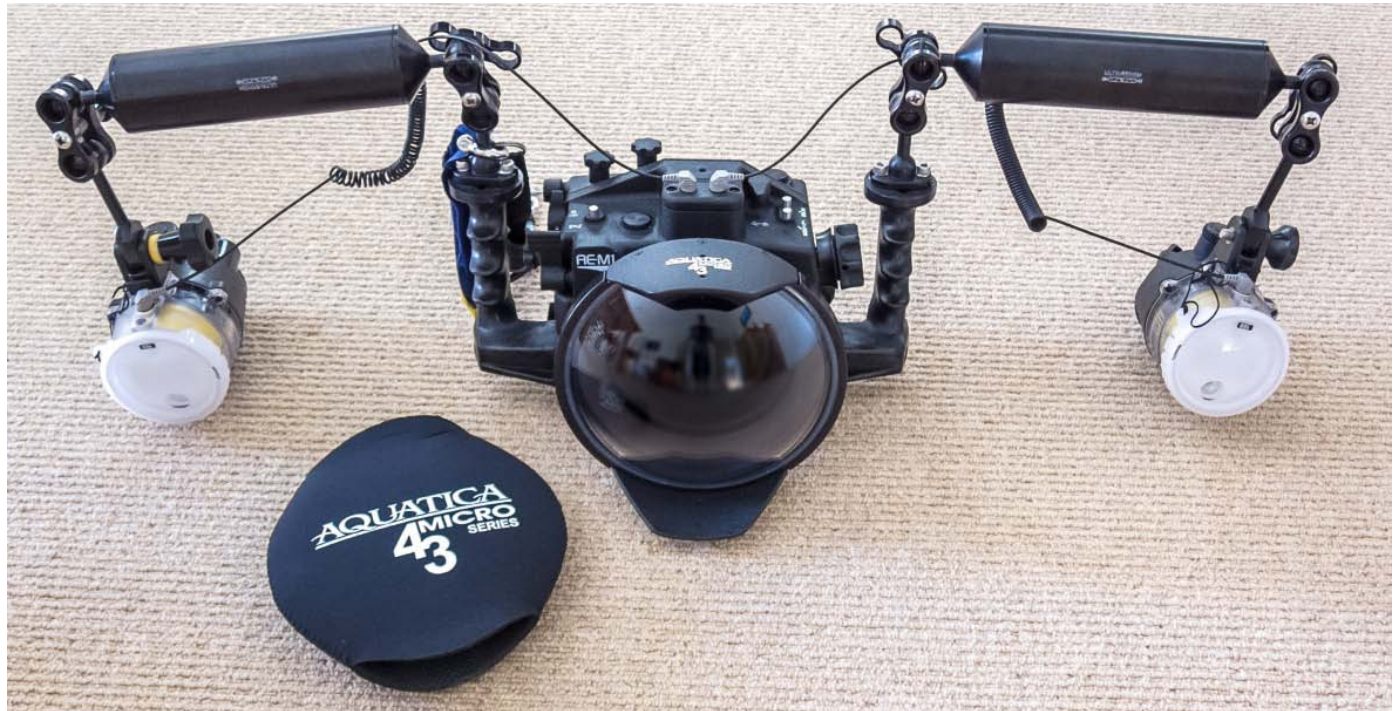
With the SW8 dome this setup is neutrally buoyant
