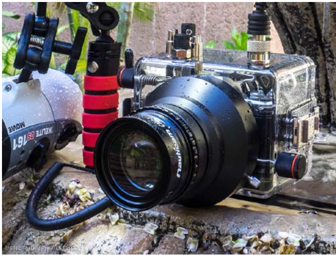
Nauticam Cmc With Spacer Mounted To Ikelite Macro Port For Panasonic 45Mm Macro.
