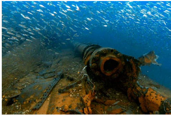
The remains of the prop shaft. Blown apart by salvage teams to access the bronze bearings. Canon 550d, Tokina 11-16mm Wide angle lens, Sea&sea YS-D1 Strobos(x2), Aquatica housing, 8in Dome f/9, 1/60, ISO400, 11mm
