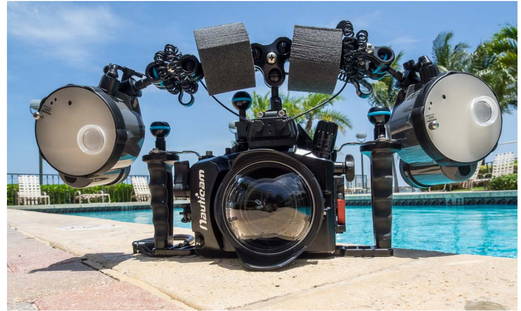
Nauticam NA-EM1 housing with Zen DP100 port and Panasonic 8mm fisheye using two Inon Z-240 strobes
