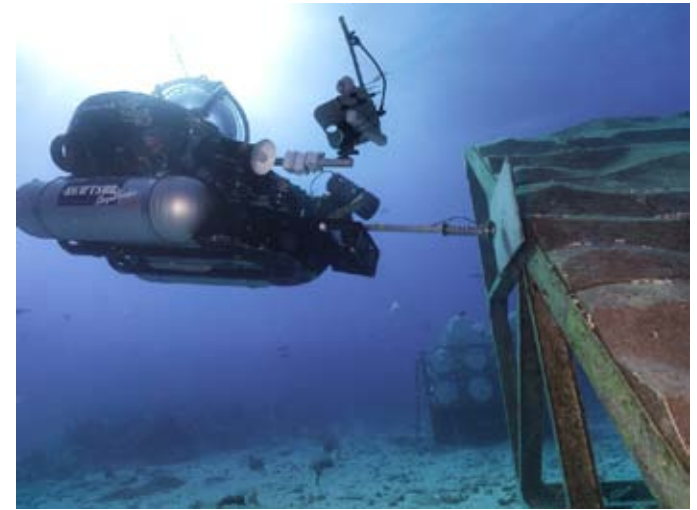
Sub Docking was achieved by an electromagnet and an iron plate. Pilot is Mike Gernhardt, a four Space Shuttle Flight Veteran. Asteroids may have sufficient iron content to allow for this type of attachment. Hasselblad H3DII-°©_31 ISO 200 f/4 1/350.
