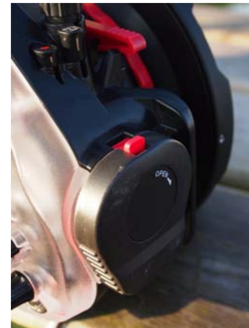
A single cam lock secures the case without removing finger nails
