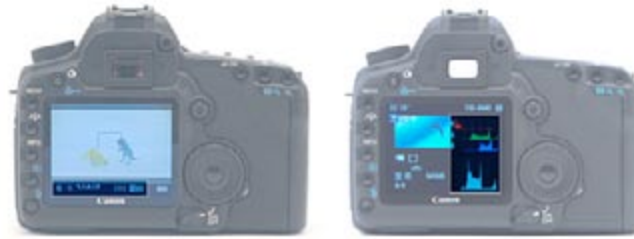
In video mode, your f-stop and shutter speed values are displayed at the bottom of the LCD. To determine best exposure, shoot a test clip (or photo) and check the three channel histogram display in playback mode.
