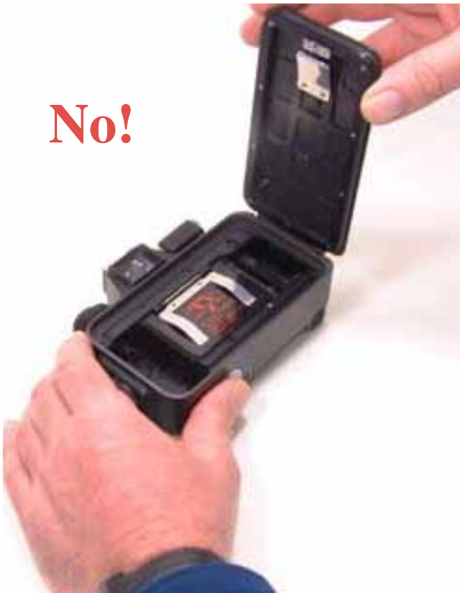
Opening a Nikonos V like this could allow water to drop into the camera around the frame counter assembly
