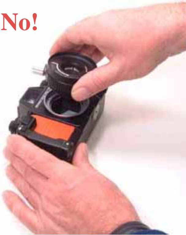
Never remove a lens like this as water droplets can fall into the throat of the camera and get onto the shutter blades
