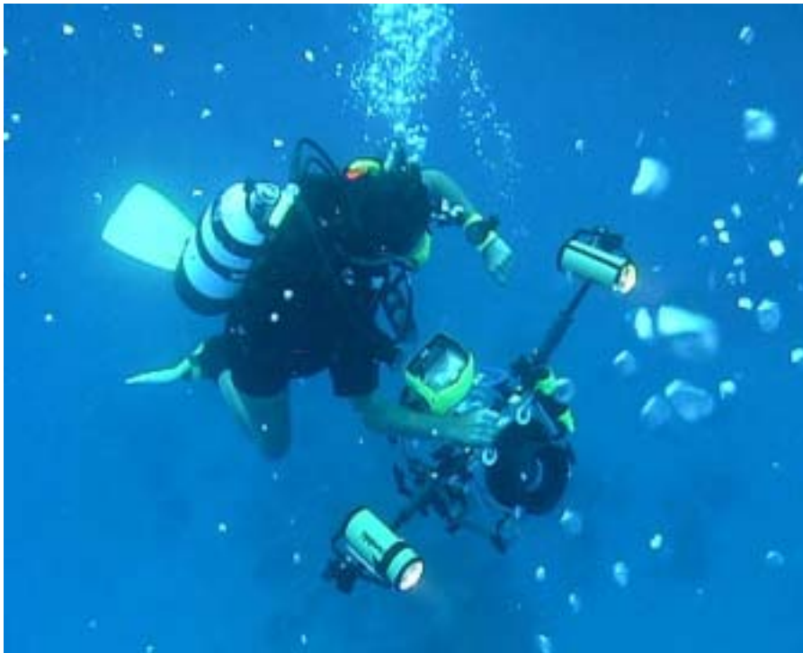
Dolly at 5m stop, lights on extended top-mount arms, dome port for wide angle.
