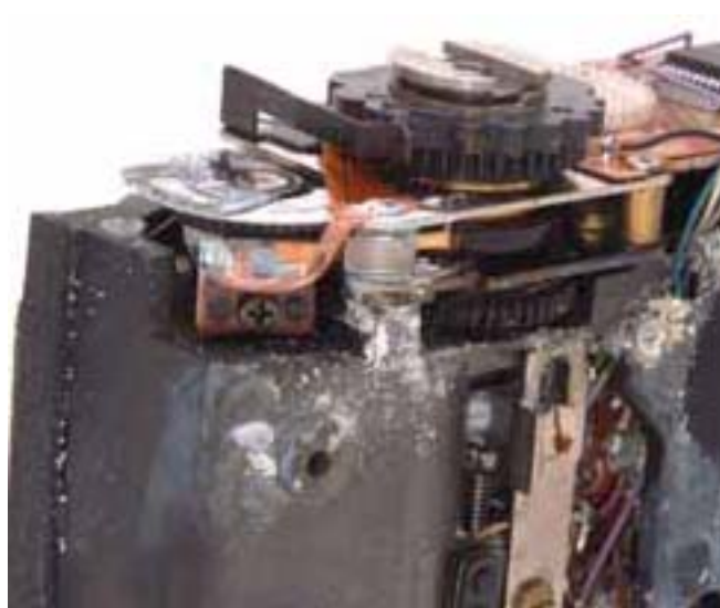
Corrosion can clearly be seen around the frame counter assembly which also contains the main power contacts.
