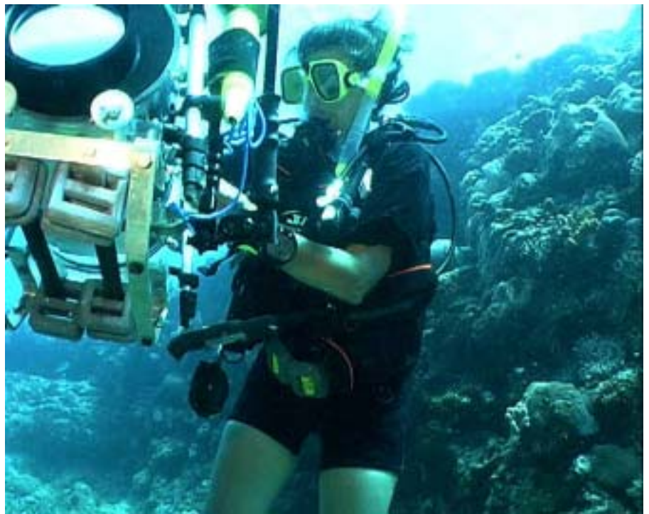
Dolly in mid water, shows weights beneath camera on rails - depth 8m.
