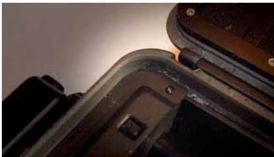
Tell tale signs of corrosion . If you open the back with the camera pointing down, there is a strong chance that water will drop into the camera
