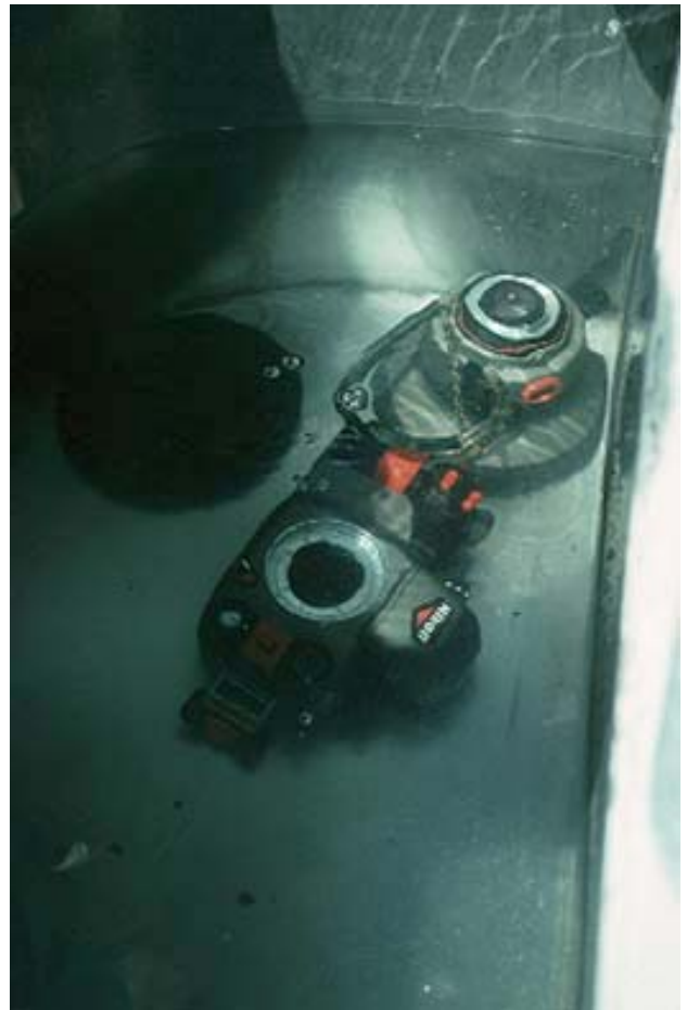
Never remove a lens like this as water droplets can fall into the throat of the camera and get onto the shutter blades
