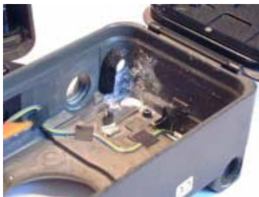
Tell tale signs of corrosion . If you open the back with the camera pointing down, there is a strong chance that water will drop into the camera
