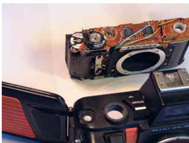
The inner body of a Nikonos V is a very snug fit in the main outer body. This keeps the camera small but any slight amount of water getting into the camera will cause problems with the electronics and mechanics
