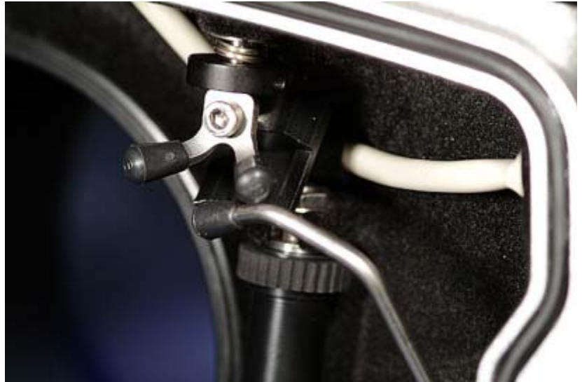
Seacam uses an ingenious double-wiper system to access two buttons from one control. The photo above shows the control inside the housing for the Flash and Exposure Compensation.
