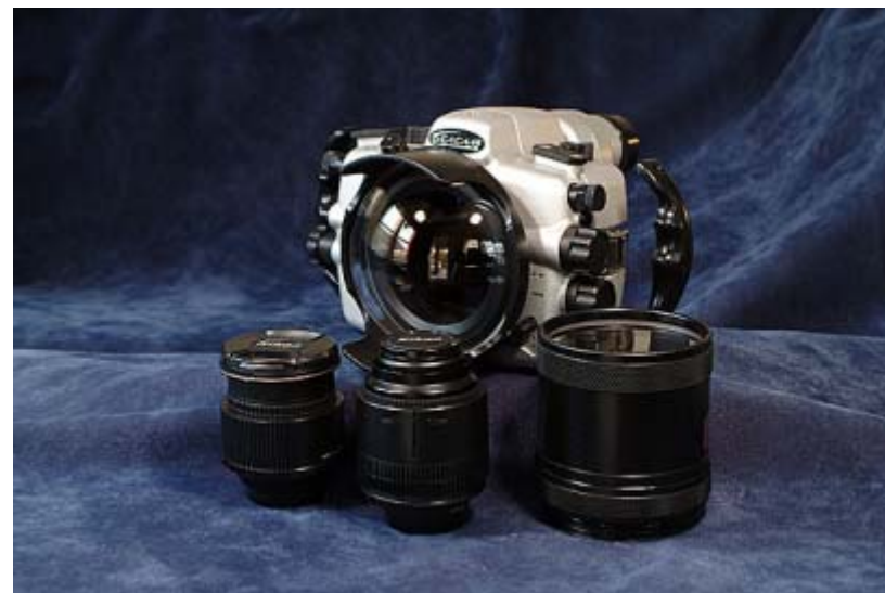
The 12-24DX with zoom gear, the 105mm with focus and AF/MF Shift collar, and the flat port with extension ring. The flat port and extension for the 105. Unlike other manufacturers, Seacam puts the focus and AF/MF shift controls on the housing
