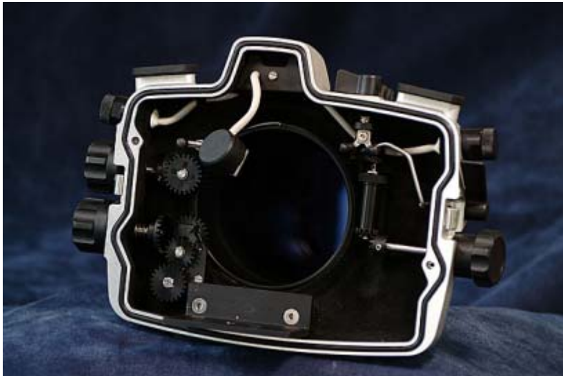
The housing front, showing the mounting tray.
