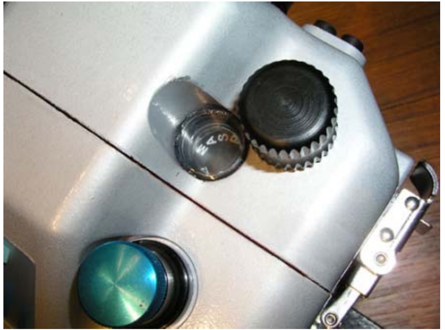
One excellent feature of the Jonah housing is the clear panel which allows you to see the mode dial setting. Photo by Craig Jones.
