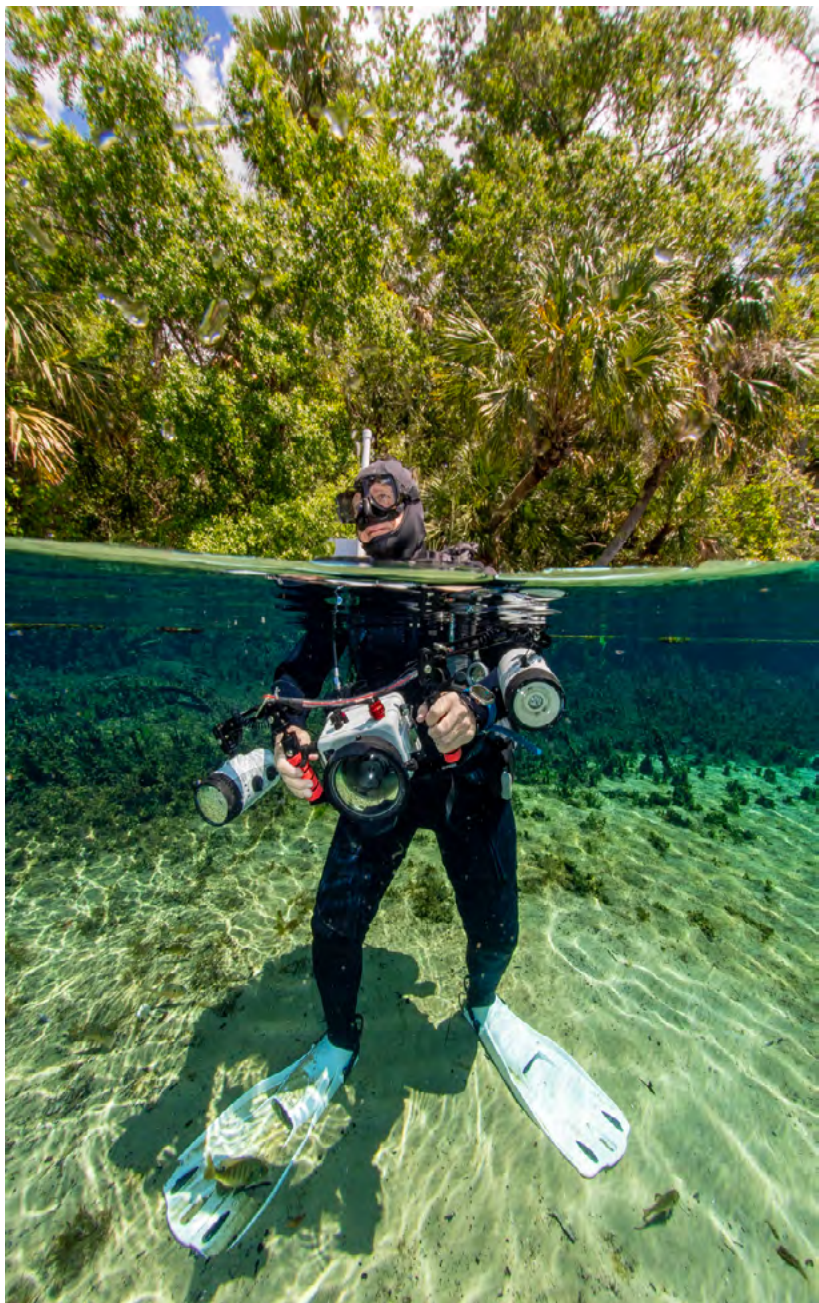
Diver Dave, Sony A7C II, Sigma 15mm F/2.8, 140mm dome, Marelux housing, Apollo S strobes with yellow diffusers, ISO-640, F/22, 1/160th sec
