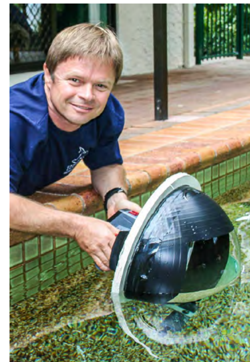
This 14" dome was initially built for a Seacam housing then converted to a Subeye Reflex with an 18mm lens
