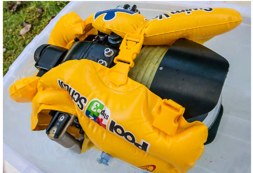
A child's life jacket can be used to float the housing at precisely the right depth. Here my D800 housing also has a foam buoyancy collar around the port extension
