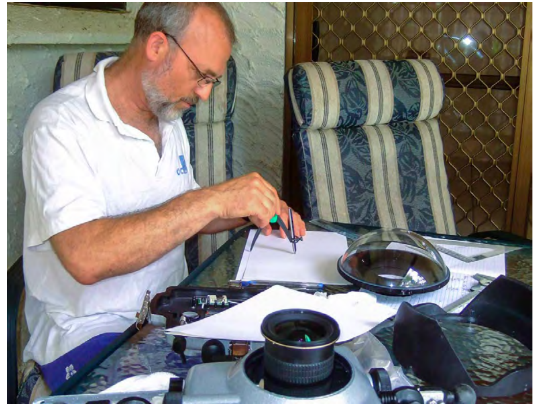
Darryl Torckler making a pattern to measure the radius of one of his dome ports
