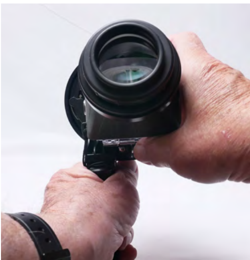
(Top left) The grey knurled button is well placed to release the lens with a 90° turn (Left) The two handed handling produced steady footage
