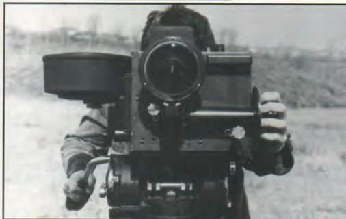
(Left and below) The IMAX camera was not the easiest of cameras to put in a housing and the first version leaked under pressure. This initial setback was resolved and an exciting compilation of underwater footage was shot. The combination of big screen and 6 track sound brought the whole show alive and made up for any lack of story or continuity.
