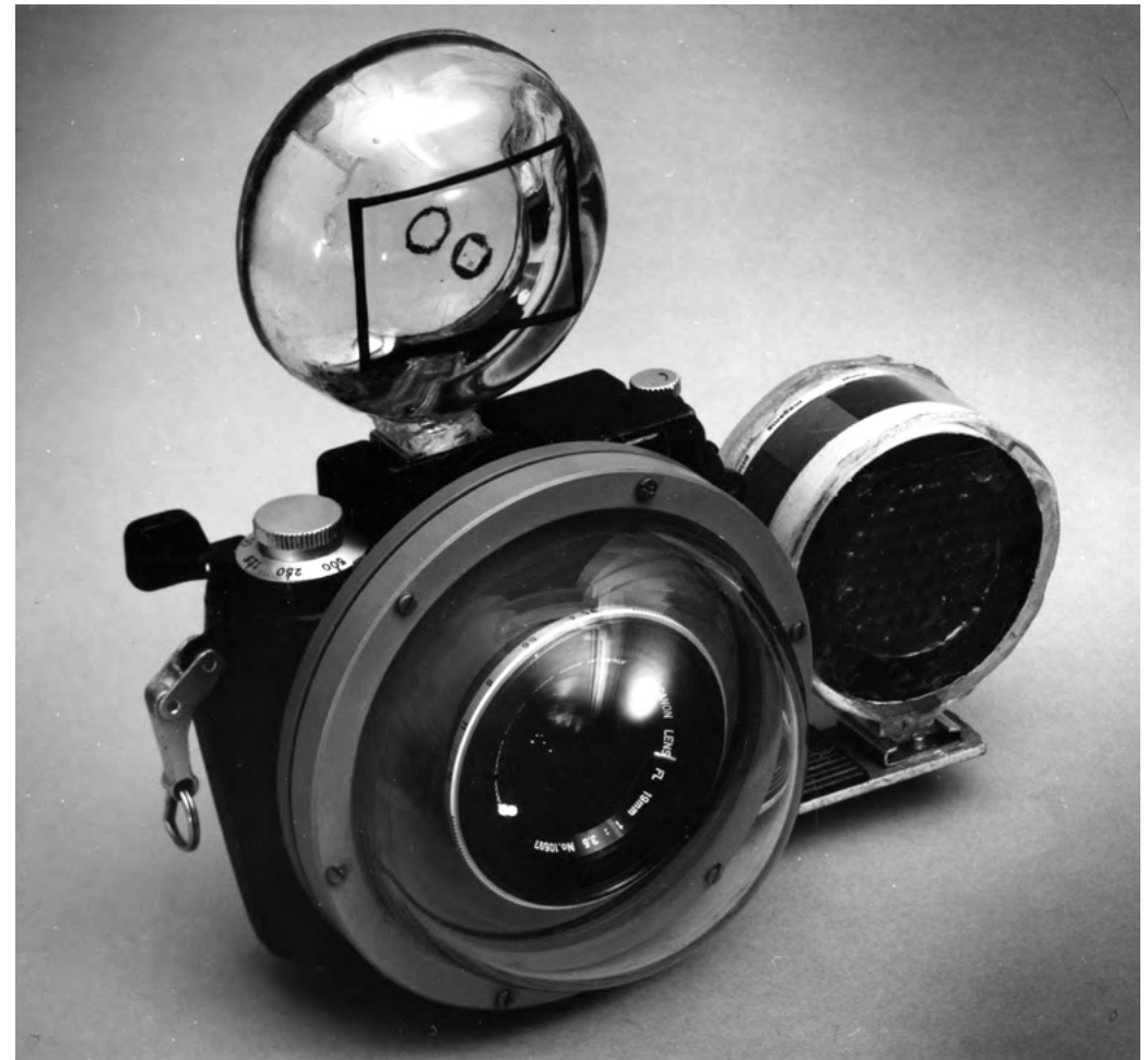
Nikonos 1 with Canon FL19mm f:3.5 Lens in Pat Baker Dome-Ported Mount
