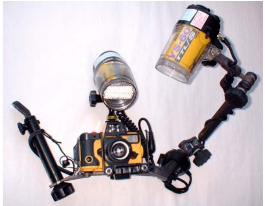
All of the macro images in this article were shot using the Sea & Sea MotorMarine II-EX with either a Macro Lens 2T (1:2) or 3T (1:3) conversion lens. Illumination was provided by dual Sea & Sea YS-60TTL S strobes synchronized with a 4 Pin Dual Sync Connect, mounted using Sea & Sea's Hot Shoe Arm and Sea Arm V. A Sea Arm IV was used as a handle for carrying the system.
