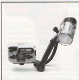
The YS 50MS is supplied complete with arm and baseplate. At the rear of the housing, the control switch and ready light port are situated. The battery cover needs to be pushed home firmly as a positive pressure builds up in the sealed battery compartment.
