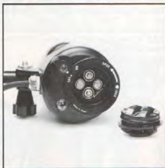
The YS 50MS is supplied complete with arm and baseplate. At the rear of the housing, the control switch and ready light port are situated. The battery cover needs to be pushed home firmly as a positive pressure builds up in the sealed battery compartment.
