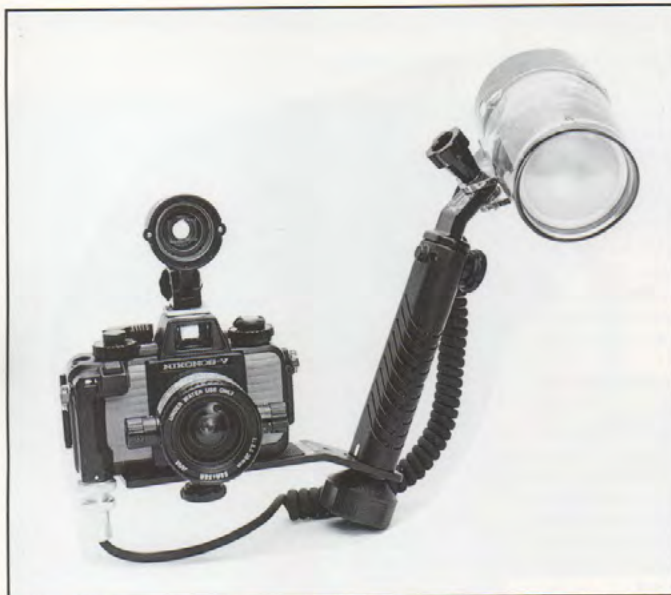
The YS 50TTL is the least expensive TTL flash currently available. The arm extends to double the flash to lens distance and a double bracket is available to mount a YS 50MS set to slave on the right of the camera.
