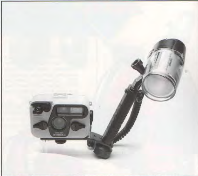
The YS 50MS is supplied complete with arm and baseplate. At the rear of the housing, the control switch and ready light port are situated. The battery cover needs to be pushed home firmly as a positive pressure builds up in the sealed battery compartment.
