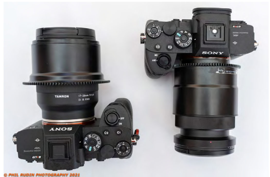
Tamron 17-28mm F/2.8 left, Sony FE 16-35mm F/4 right, both zoomed wide, both with Nauticam gears, Sony A7R IV bodies. Notice the extension at the 16mm on the Sony v. the Tamron at 17mm.
