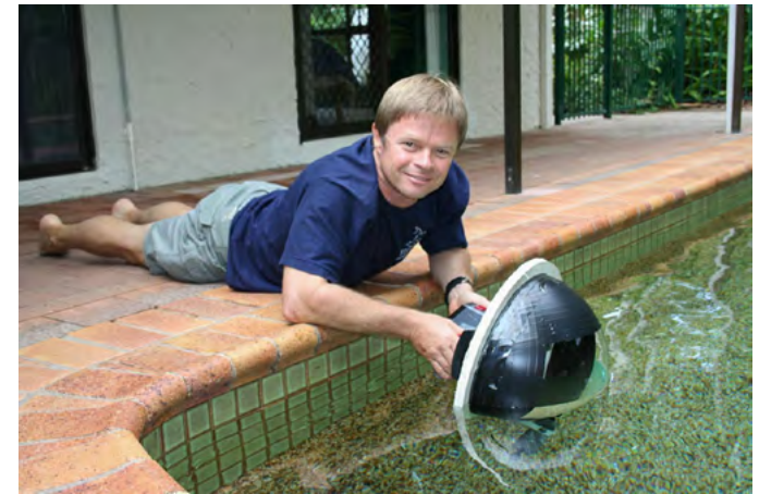
The 14" (36cm) dome made for an 18mm lens on the Subeye Reflex then converted to the Seacam D200 housing
