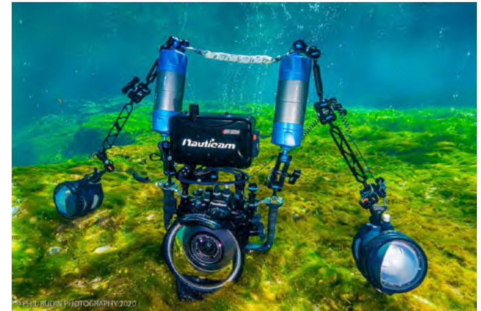
Housing System waiting for testing, Ginnie Springs, Florida, Aquatica A7rIV Pro Housing, Sony A7R IV, Two Inon-Z330 strobes, Rokinon 14mm F/2.8 AF, with Aquatica 200mm Acrylic Dome Port, ISO320, F/14, 1/15th sec
