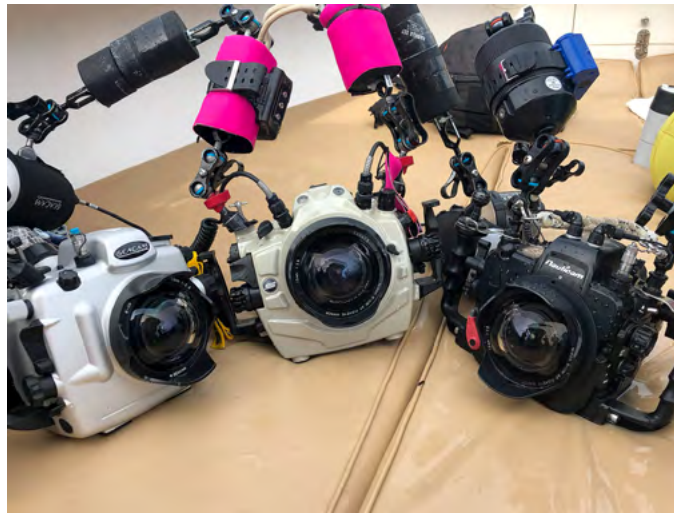
The Nikonos 13mm fisheye is a water contact autofocus lens from the Nikonos RS. It can be reprogrammed to work with modern Nikon SLRs – here mounted on Seacam, Subal and Nauticam housings on my La Paz workshop.
