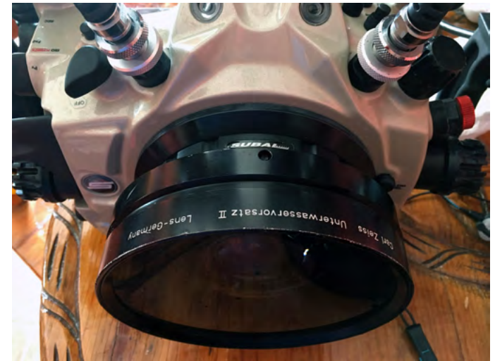
The Carl Zeiss "Unterwasservorsatz" optical corrector port, with a Nikon 20mm AF attached to my Subal housing, giving a rectilinear FOV of 94°.
