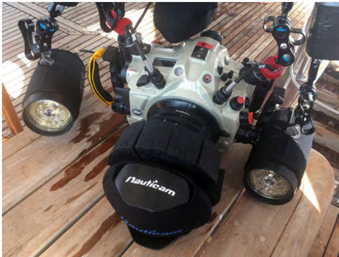
The Nauticam WACP and Nikon 28-70mm attached to my Subal housing. With a Nikon FX camera this gives a underwater corrected fisheye with a FOV from 130° to 57°.
